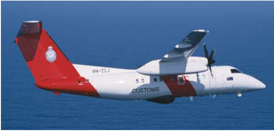
The NAS Dash 8s will be fitted with a Raytheon SV2022 search radar. (NAS)
